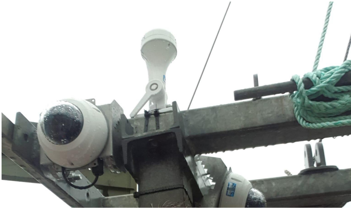
Figure 3: CCTV cameras and GPS fitted on one of the participating vessels.
